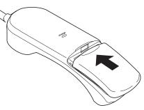
**Note:** The built-in Memory Backup feature allows up to 3 minutes to disconnect the old battery pack and install a new one without losing any numbers stored in memory.
